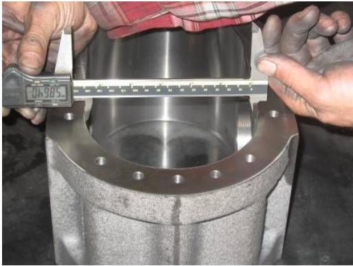
Housing Measurement Location.
